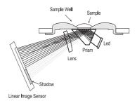
In the **HI 96821** refractometer, light from an LED passes through a prism in contact with the sample. An image sensor determines the critical angle at which the light is no longer refracted through the sample.
