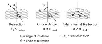
The critical angle can be used to easily calculate the refractive index according to the equation:
